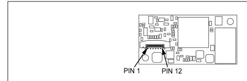
Figure 35. Decode Board (TTL) Output Connector
